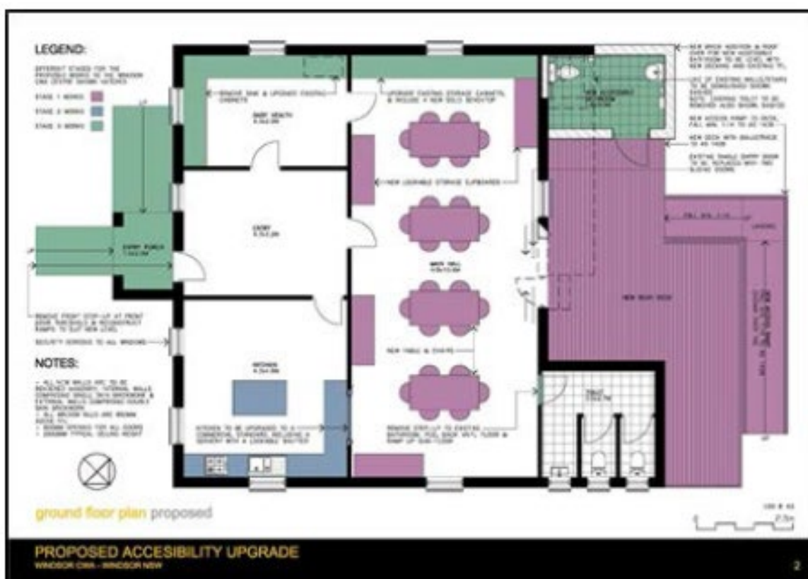
Figure 9 CWA Building – Proposed Accessibility Upgrade (Sourced from the McQuade Park Plan of Management November 2022; Page 39)
