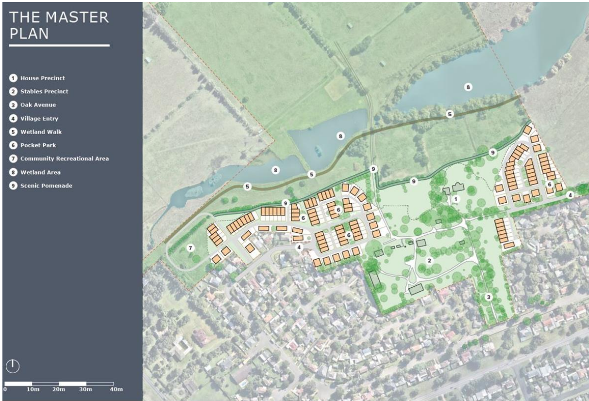
Figure 6.1 Extract from the proposed Hobartville masterplan showing heritage buildings (red) and proposed townhouses and cottages (yellow). (Source: Roberts Day)
