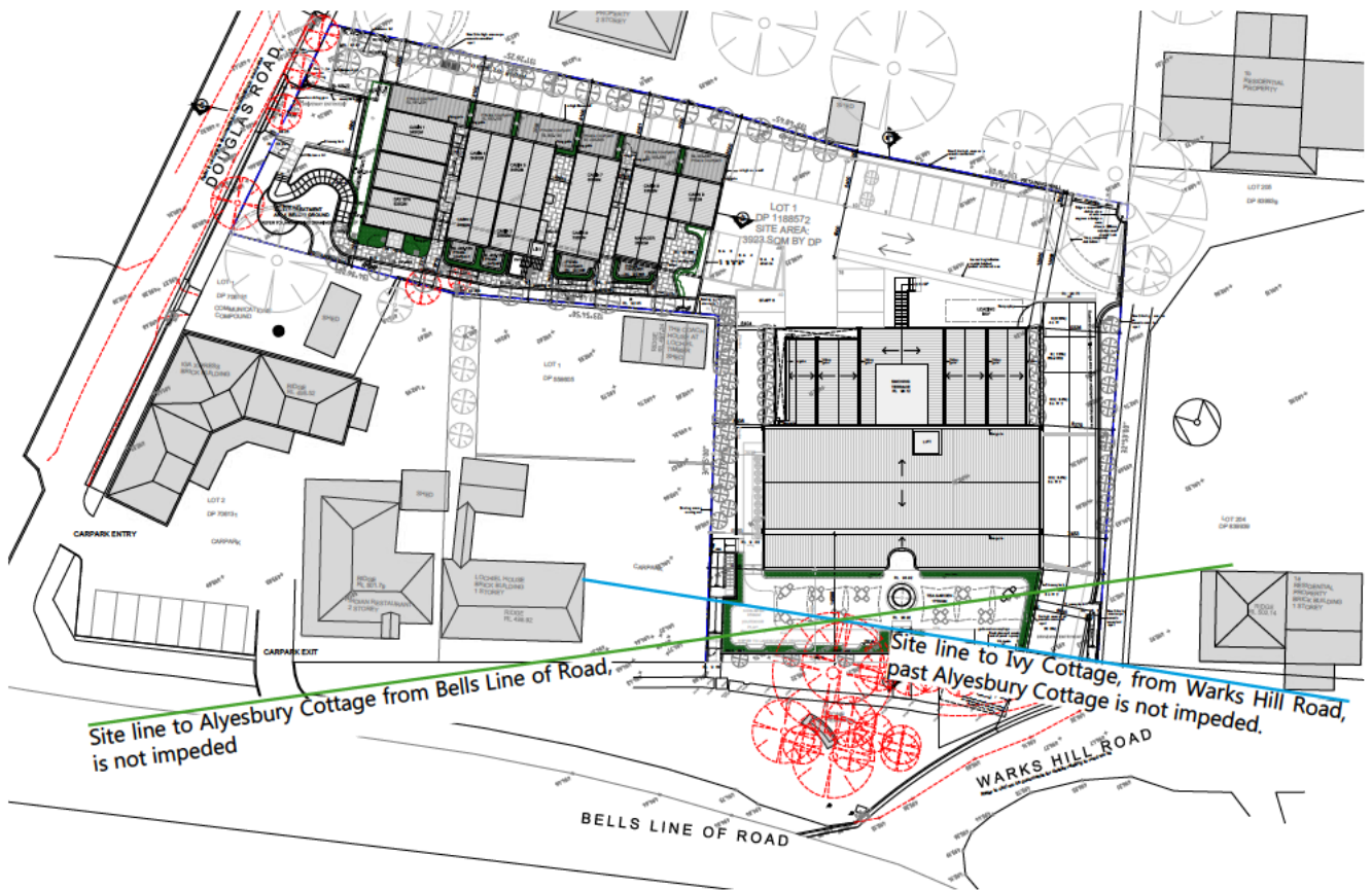
Figure 6.6 (above) Proposed Site Plan, with overlay showing view corridors to neighbouring heritage items. Source: Archibiosis Architects, Kurralong Heights Hotel and Accommodation, Proposed Site Plan, SK101, Issue 1, 17/13/22 (not to scale)
