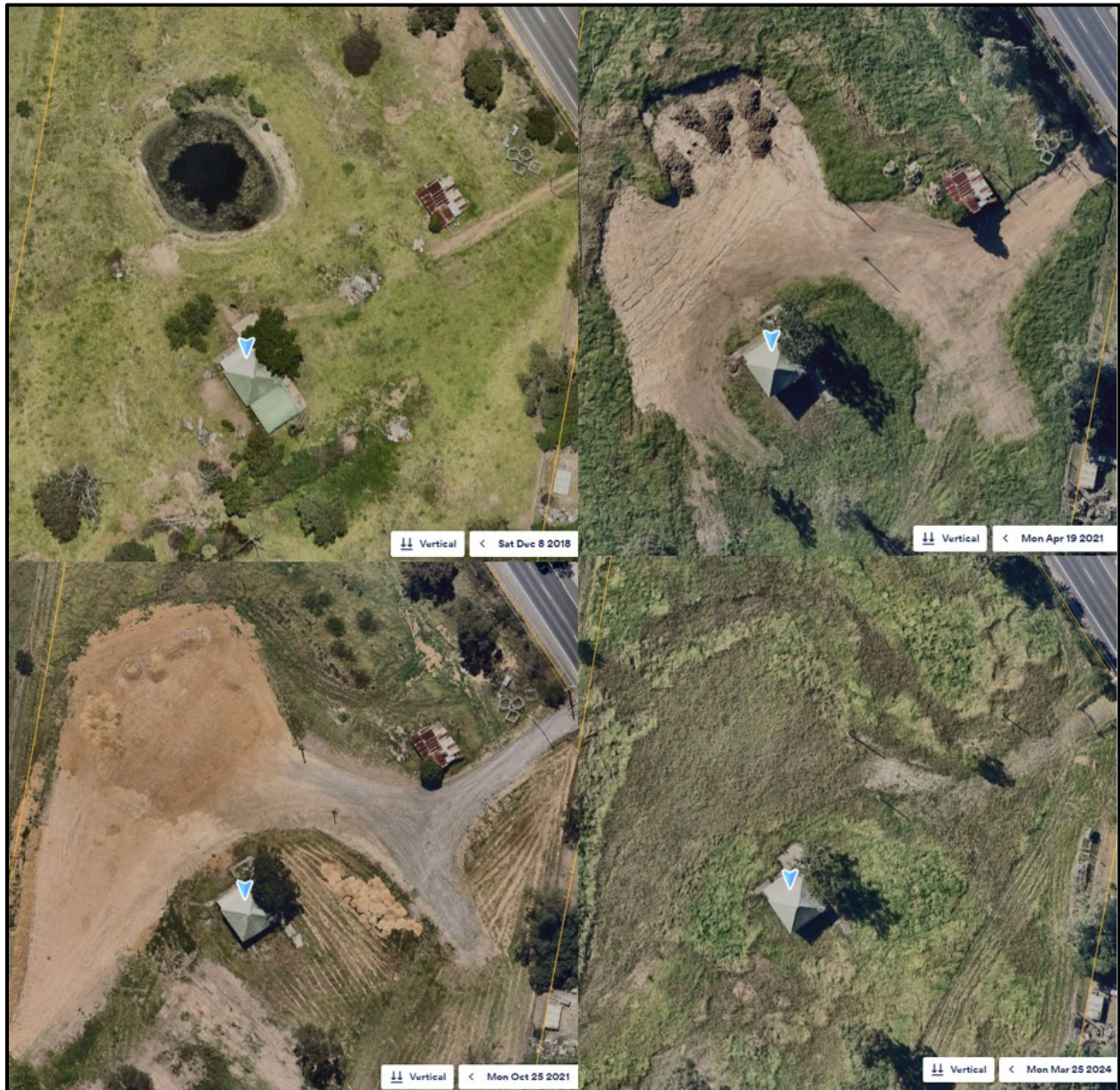
Figure 6. Aerial imagery demonstrating the decommissioning of the dam.
